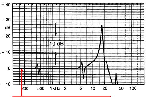
Calibration at 159.2 Hz will not show the damage directly!
